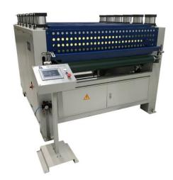
The first upper pressing roller is motorized to assure the floorboards are fed in without any problem. The other 5 upper rollers are free driven.
