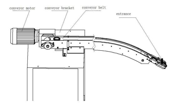
This part of the conveyor belt is mounted in the conveying holder, Conveyor belt forward by the motor driven, when ring drops from the processing ring portion onto the conveyor belt, it will transfer at the entrance, then jaw blocked by parked and waiting for the bottle to pull. The conveyor belt has remained rotation ensure the ring continued feeding.
