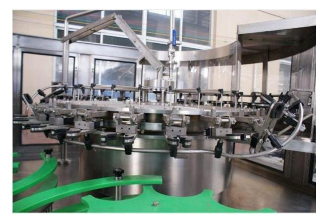
USE conveying screw into the bottle and the bottle into the thumbwheel direct-connect technology, by the bottle feeding steel thumbwheel sent directly to the washing bottle machine. The bottle transmission are all made of palm technology, transform bottle shape does not need to adjust equipment, only need to replace the arc guide plate, associated with the bottle diameter changing bottle shape need to replace a small amount of star wheel, arc guide plate can be realized
