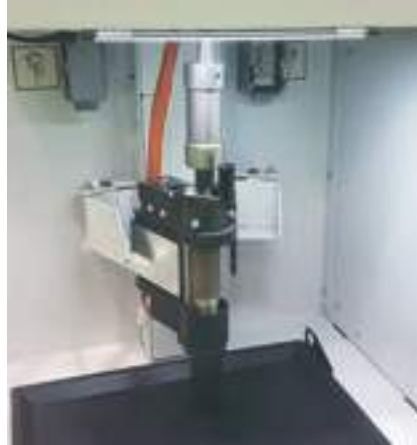
gPod, the Biesse device for polyurethane glue with "PUR on demand" system for melting only the required amount of glue in real time.
