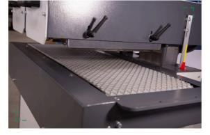
**Professional rubber feed belt** A gray feed belt of the highest category is used to pull the material.
