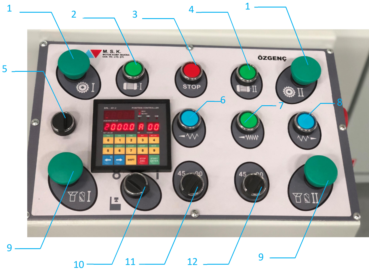
Control panel with position controller device
