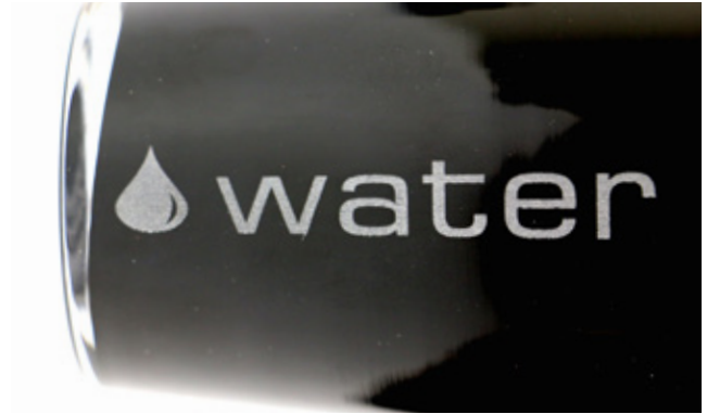
Laser engraved drinking glass with rotary device
