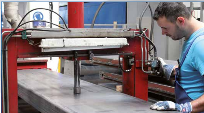
Option "Lowering Device": After welding, the runways for wheel alignment lifts are straightened exactly flat in the area of the turntables and sliding plates.
