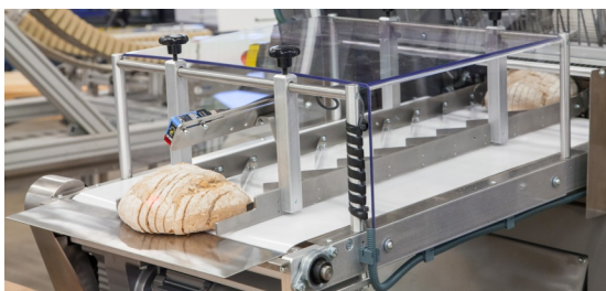
Band conveyor outlet
