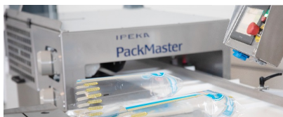
Bag pre-opening with air blow
