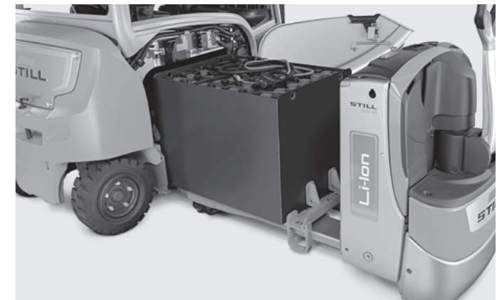
Battery change with electric pallet truck
