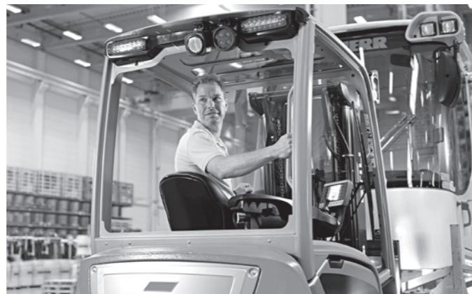
Swivel seat handle with optional horn operation for ergonomic reverse driving
