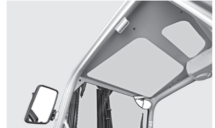
Enhanced visibility thanks to panoramic armoured glass pane
