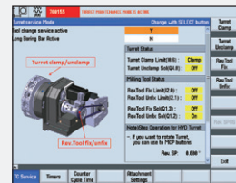
Maintenance and service convenience function Maintenance and service of major units and peripheral devices, timer setting and parts counter setting can be easily carried out on a convenient screen.
