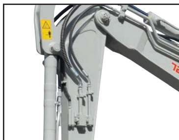
Auxiliary Hydraulic Lines
