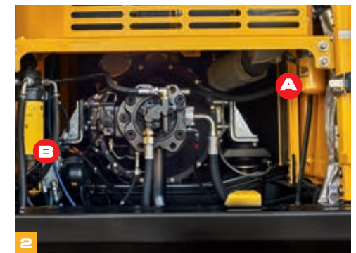
(A) Hydraulics oil filters (B) Fuel filters
