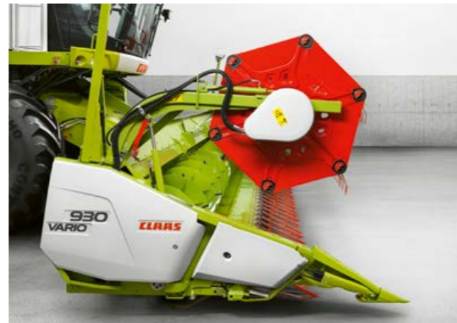
Cutterbar table retracted – grain (- 100 mm).
