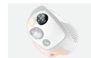
The CMOTION multifunction control lever is used to adjust reel parameters (reel height, reel level) and the snapping plate distance of the maize picker.
