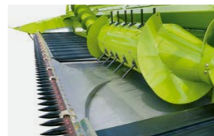
Guide element with curved track.
