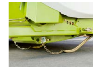
Sensor bands detect the position of the front attachment for AUTO CONTOUR and CONTOUR.
