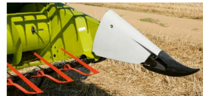
Special long or short crop dividers can deflect upwards.
