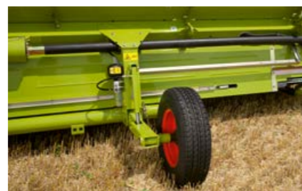
Stabiliser wheel for optimal front attachment guidance.
