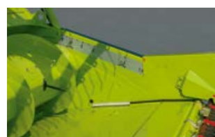
The operator in the cab has a perfect view of the position indicator for the cutterbar tray.
