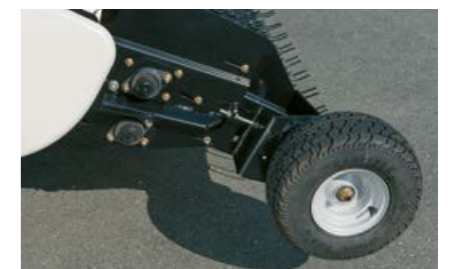
Castor guide wheels limit the depth.
