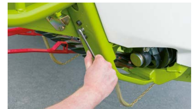
Easy adjustment of divider height using the panel key.
