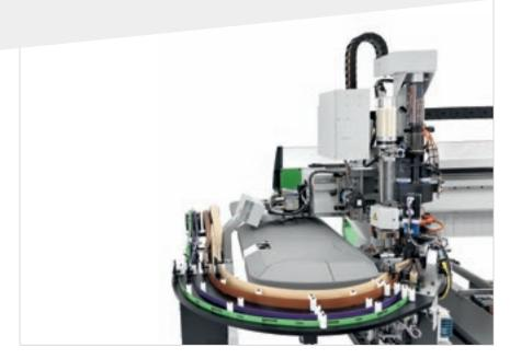
The automatic edging feeder, mounted on the X carriage, allows the user to change between thin or thicker edges during the same machining cycle.
