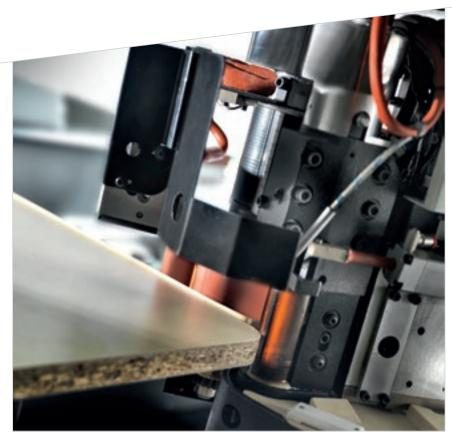
Similar to straight line edgebanding machines, **the glue is applied directly onto the panel** in order to ensure optimal adhesion quality. It supports the use of thin or transparent (3D) edges, as well as thicker and sturdier edges.
