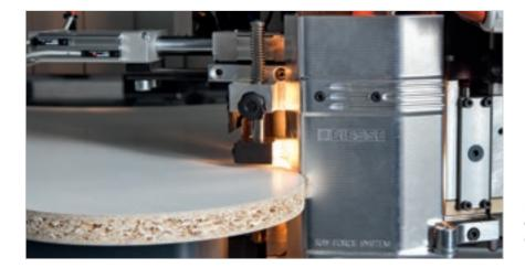
RayForceSystem equipment, interchangeable with the use of EVA or PUR glues, for the highest quality of the finished product.
