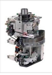
Trimming aggregate with non-stick liquid delivery.
