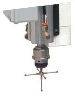
The cross-head thickness tracer enables operators to measure panel dimensions with absolute precision.
