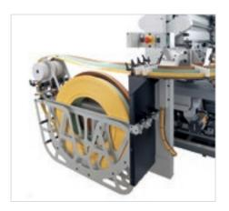
Thin or thick edges, either pre-cut or coiled, with automatic or manual feeding.
