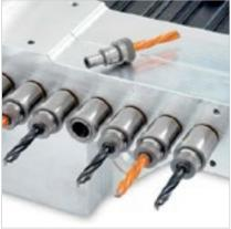
Quick and easy boring head change thanks to the exclusive spindle snap-on coupling system.
