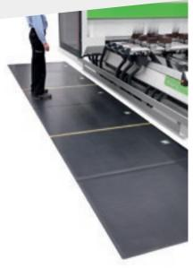
**Pressure-sensitive floor mats** enable the machine to operate at constant maximum speed.
