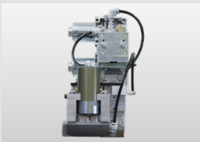
Automatic adjustment of the glue joint scraper
